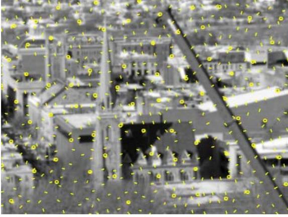
Figure 3: Example intermediate resolution driving features, which are more sparse than matchable features. Circles are corners and line segments are face points, oriented along the direction of greatest eigenvalue.
